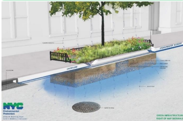
Storm water infiltration greenbelt (rain garden)
