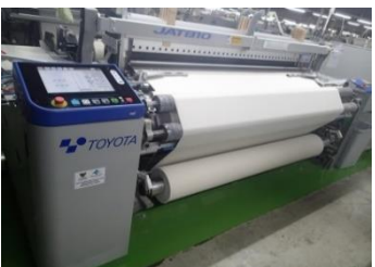
Upgrading air-saving loom at textile factory, TORAY etc., Indonesia, Thailand, and Bangladesh
