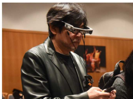
Eyeglasses-type terminal for the hearing impaired
