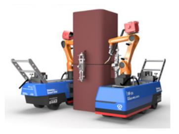
the groove with welding material. The welding work uses two robots. We also plan to introduce a non-contact system that can inspect the quality of welded components in real time.
