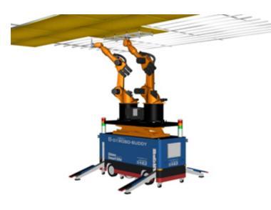
of an automatic guided vehicle. After it recognizes the location to perform the work via imaging sensors and laser sensors, it uses its two robotic arms to insert ceiling suspension bolts, assemble the base materials, and install the ceiling board, screw it into place, and install the OA floor pedestal and paneling. This robot can be used to perform multiple functions by switching the end effectors at the tip of the robotic arms.
